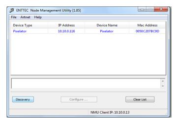
NMU (Node Management Utility) is a free Windows and Mac application that is used to manage compatible ENTTEC DMX over Ethernet nodes. NMU will not directly allow you to configure the Pixelator itself, but it can help you find your unit's IP address and then open a browser window to access Pixelator. Follow these steps:
