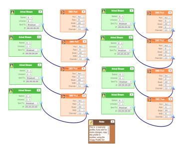
Create a new profile or edit an existing one using the profileeditor. Opens up in a new page in your web browser. Select a module on the left and the right panel will provide help about that panel. Connect a module to another using wires from one point to another.
