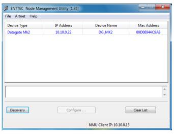
NMU (Node Management Utility) is a free Windows and OSX application that is used to manage compatible ENTTEC DMX over Ethernet nodes. NMU will not directly allow you to configure the Datagate Mk2 itself, but it can help you find your unit's IP address and then open a browser window to make the required changes. To employ the NMU, follow this set of instructions:
