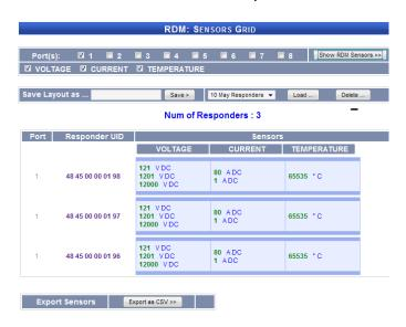
RDM Sensors page, allows discovering all RDM devices and monitoring all sensors supported by the RDM devices found. Examples include: Temperature, Current and, Voltage sensors. The displayed sensors values are refreshed, automatically every few seconds.
