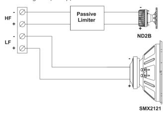
Block Diagram (passive): Standard shipping configuration
