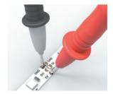
PUSH PROBES THROUGH PROTECTIVE SILICONE TO MAKE CONTACT
